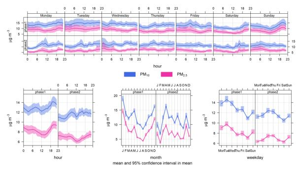
Figure 10: Temporal variations in PM<sub>10</sub> and PM<sub>2.5</sub> concentrations measured at Helsby during Phase 1 and Phase 2.
