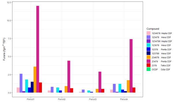
Figure 15: Furan concentrations measured at Helsby during 2020.
