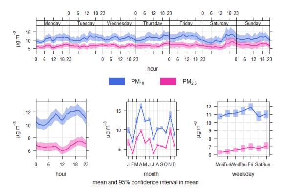
Figure 7: Temporal variations in PM<sub>10</sub> and PM<sub>2.5</sub> concentrations measured at Helsby during 2020.
