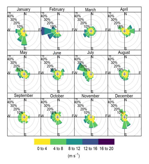
Figure 3: Monthly wind roses for Liverpool John Lennon Airport. Data source: NOAA Integrated Surface Database (ISD) (NOAA, 2020).
